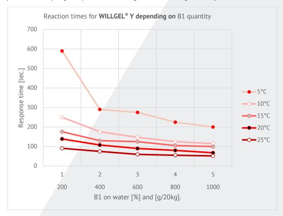
It is also possible to increase the amount of water on both sides (A and B) by a <u>maximum of</u> <u>50% to</u> obtain longer reaction times and an even lower viscosity. The final product is then weaker, but still has sufficient soil consolidation properties.
